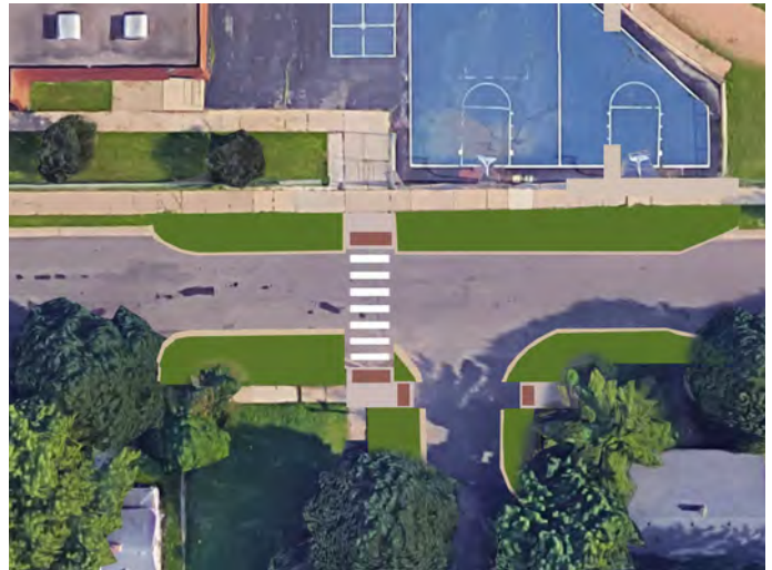
Recommendation G. Jenks Ave at Weide St. Current (left) and recommended (right). Narrowing the roadway lowers vehicular speeds and provides a shorter crossing distance for pedestrians.
