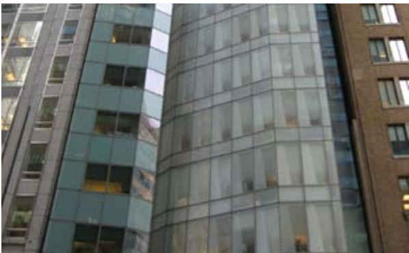
Figure 4.6 Reflect window sizes and arrangements of historic resources. In addition, consider the horizontal alignments with a historic resource.
