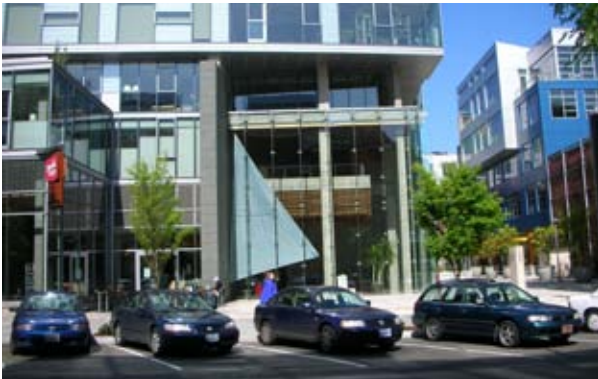
Figure 4.14 Design a new building(s) to have a high amount of transparency at the street edge.
