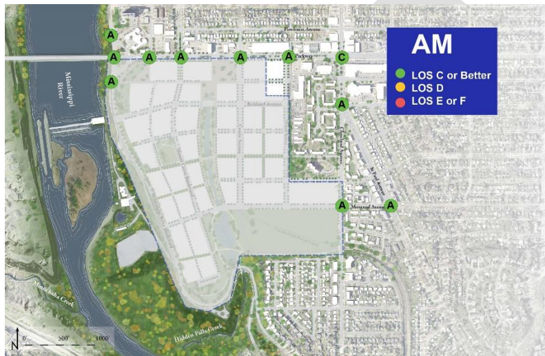
Figure 4-7: Existing conditions AM peak hour LOS
