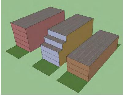
RM2 zoned property. The graphic to the left shows a rear view of buildings with a 30 ft height (A), 30 ft at rear setback with an additional foot of height for each foot of setback (B), and at the current allowed maximum height of 50 feet (C).
