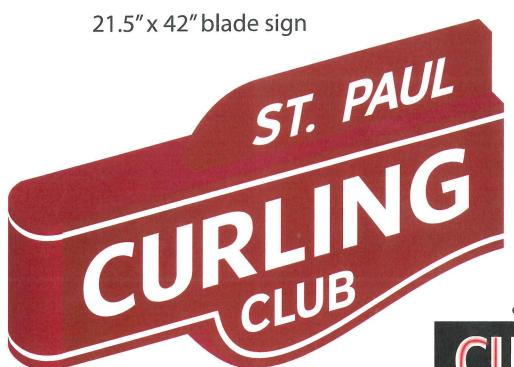
.125 aluminum constructed can 6.25" tall letters Red enamel paint White vinyl graphics Red neon tube glass in "CURLING" Double sided blade sign
