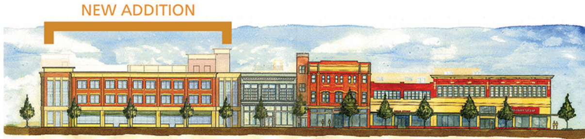
Figure 22. The proposed new addition is compatible with the historic buildings that remain on the block. Its design with multiple storefronts helps break up the mass.
