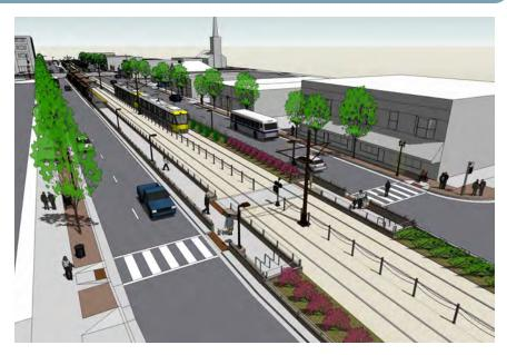
This illustration shows how non-signalized cross streets will not allow through traffic after the train is operational.
