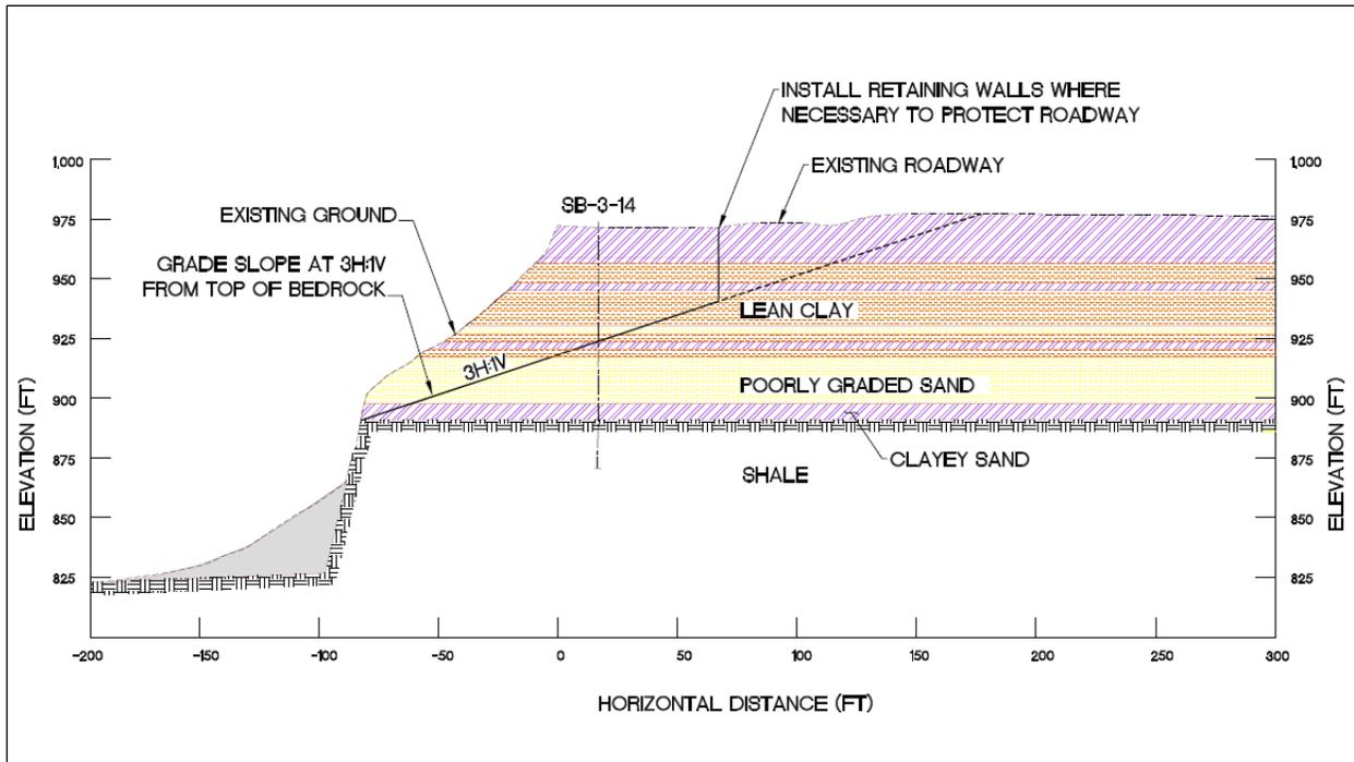
**Figure 5-2** Conceptual example of grading to a stable slope and installing a sheetpile wall to protect the roadway
