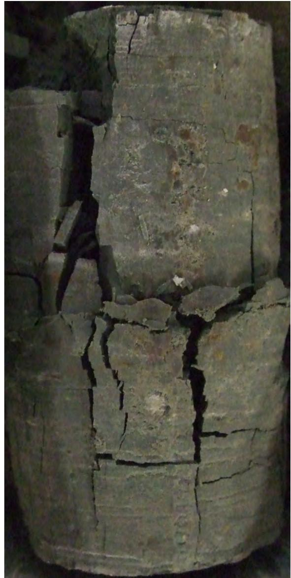
**Unconfined Compressive Strength of Intact Rock** (ASTM:D7012) Method C
