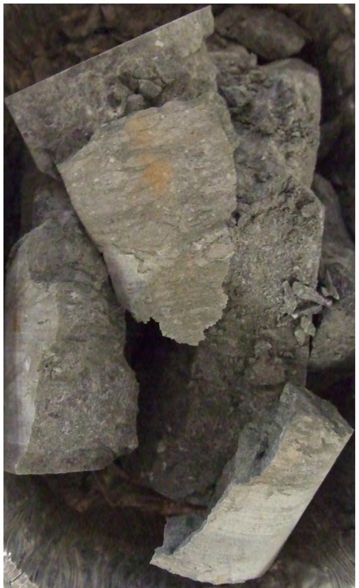
**Unconfined Compressive Strength of Intact Rock** (ASTM:D7012) Method C
