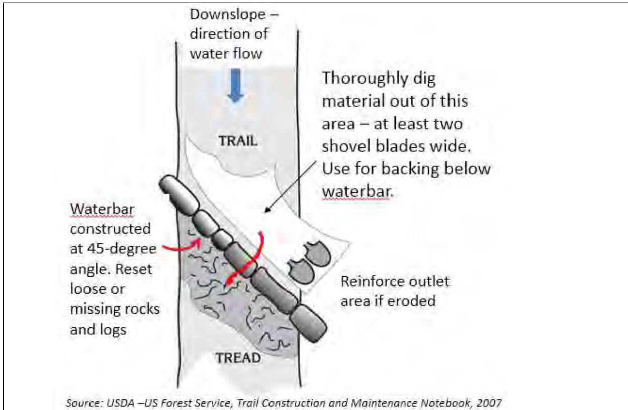
Figure 5-1 Conceptual drawing of a waterbar
