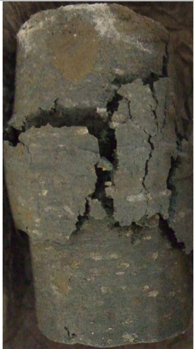
**Unconfined Compressive Strength of Intact Rock** (ASTM:D7012) Method C
