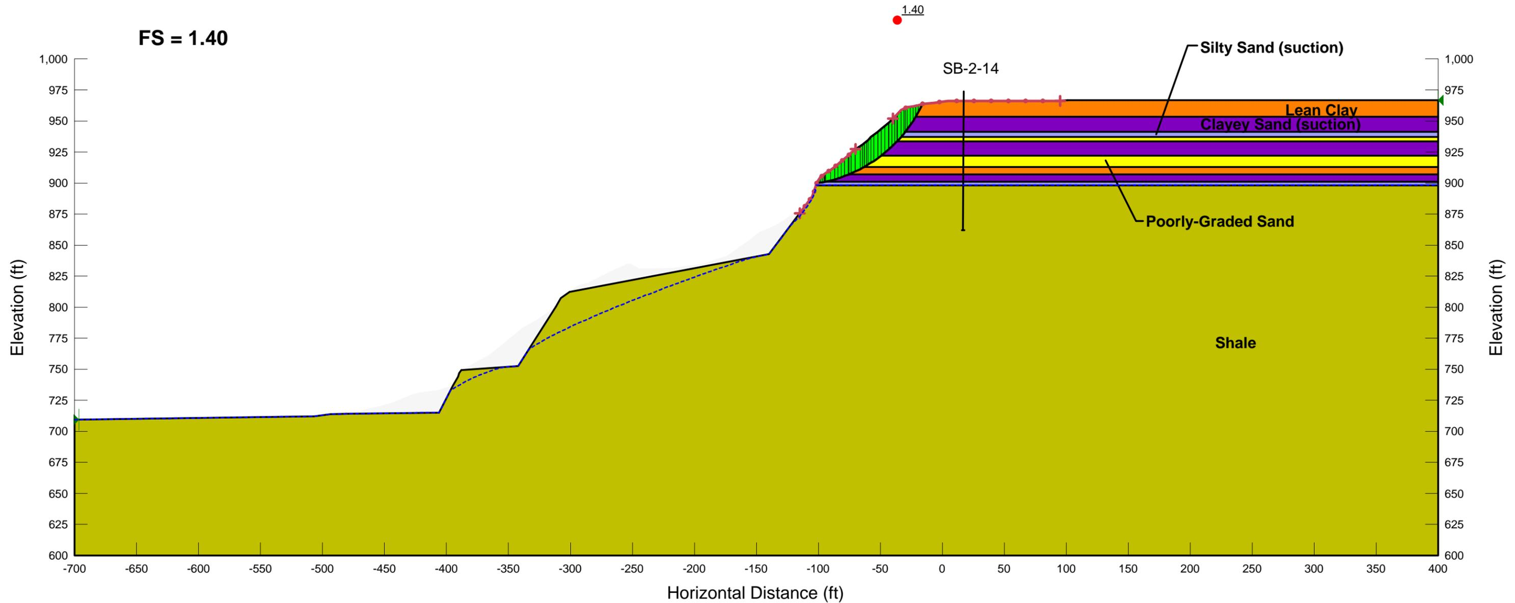
**Figure E-4 North End Drained Friction Angle with Rainfal**
