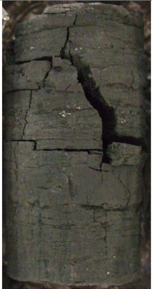
**Unconfined Compressive Strength of Intact Rock** (ASTM:D7012) Method C
