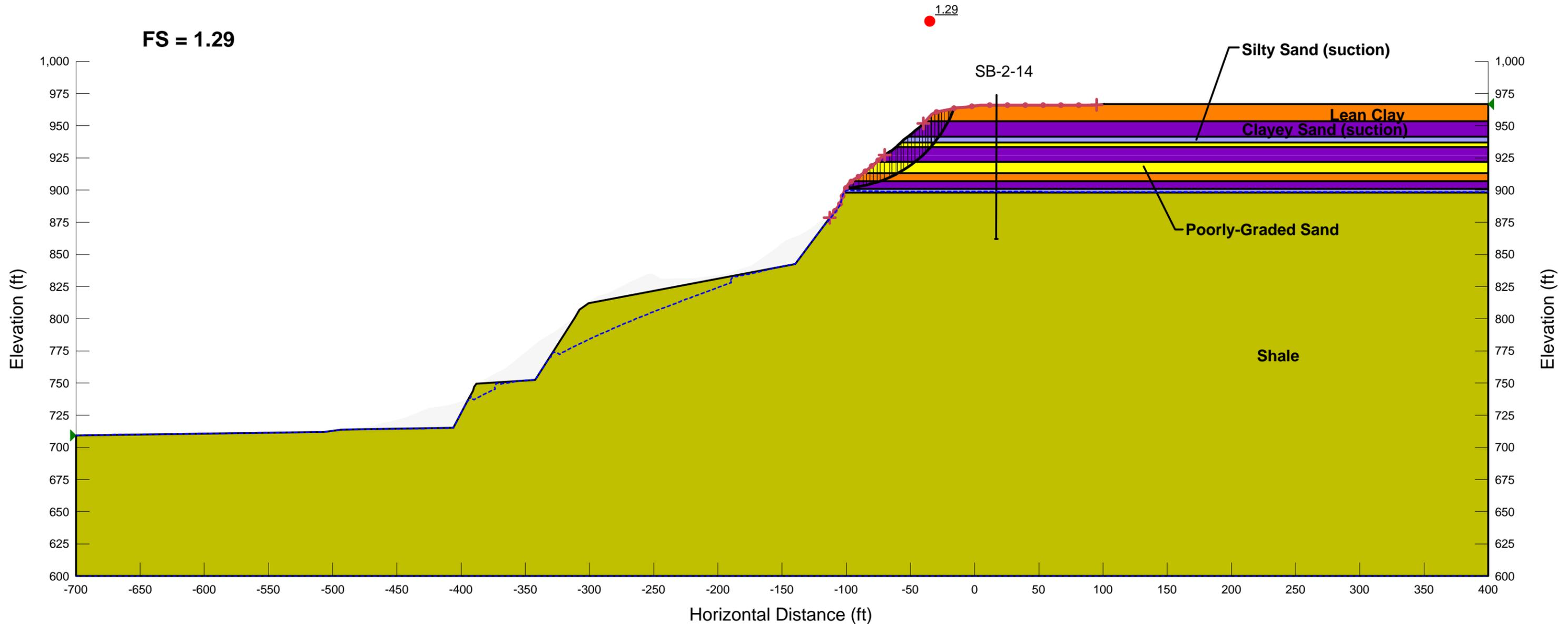
**Figure E-6 North End Drained Friction Angle with Suction with High Groundwater**
