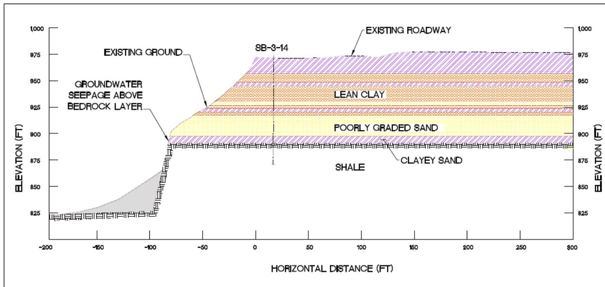
**Figure 3-1 Middle Clay Pit modeling cross section showing stratigraphy**
