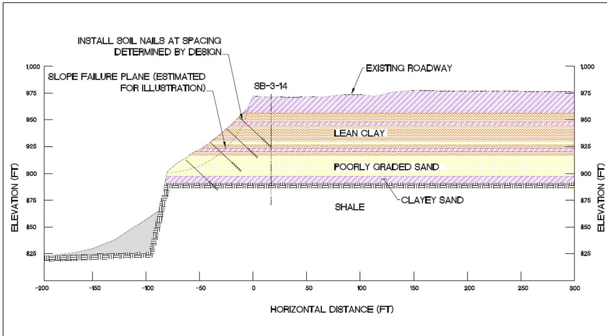
**Figure 5-3** Conceptual example of soil nailing
