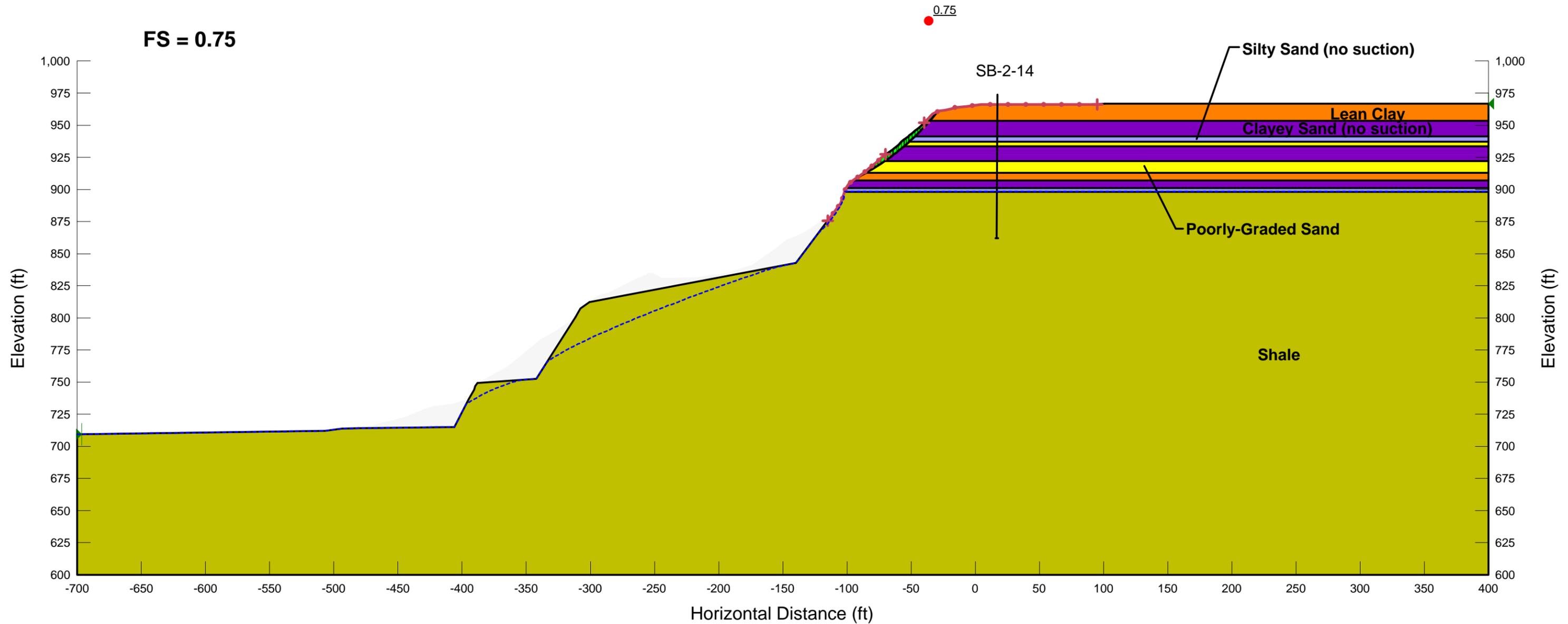
**Figure E-2 North End Drained Friction Angle at Stability**
