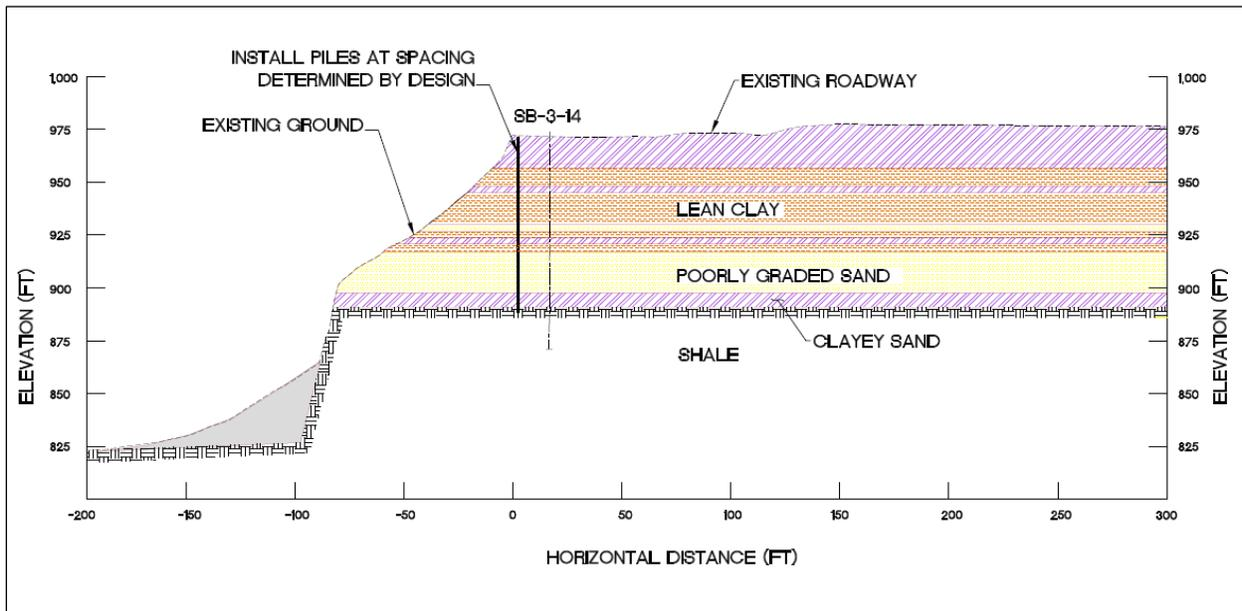
**Figure 5-4** Conceptual example of soldier piling
