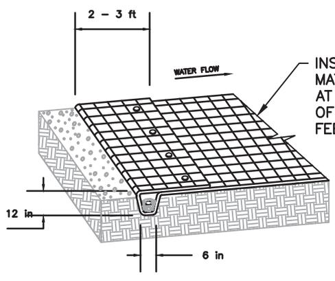
INSTALLATION DETAIL FOR MATERIAL KEYED-TRENCHES, AT THE TOP, SIDES, BOTTOM OF THE SWALE AND EVERY 25 FEET IN THE SWALE TRENCH
