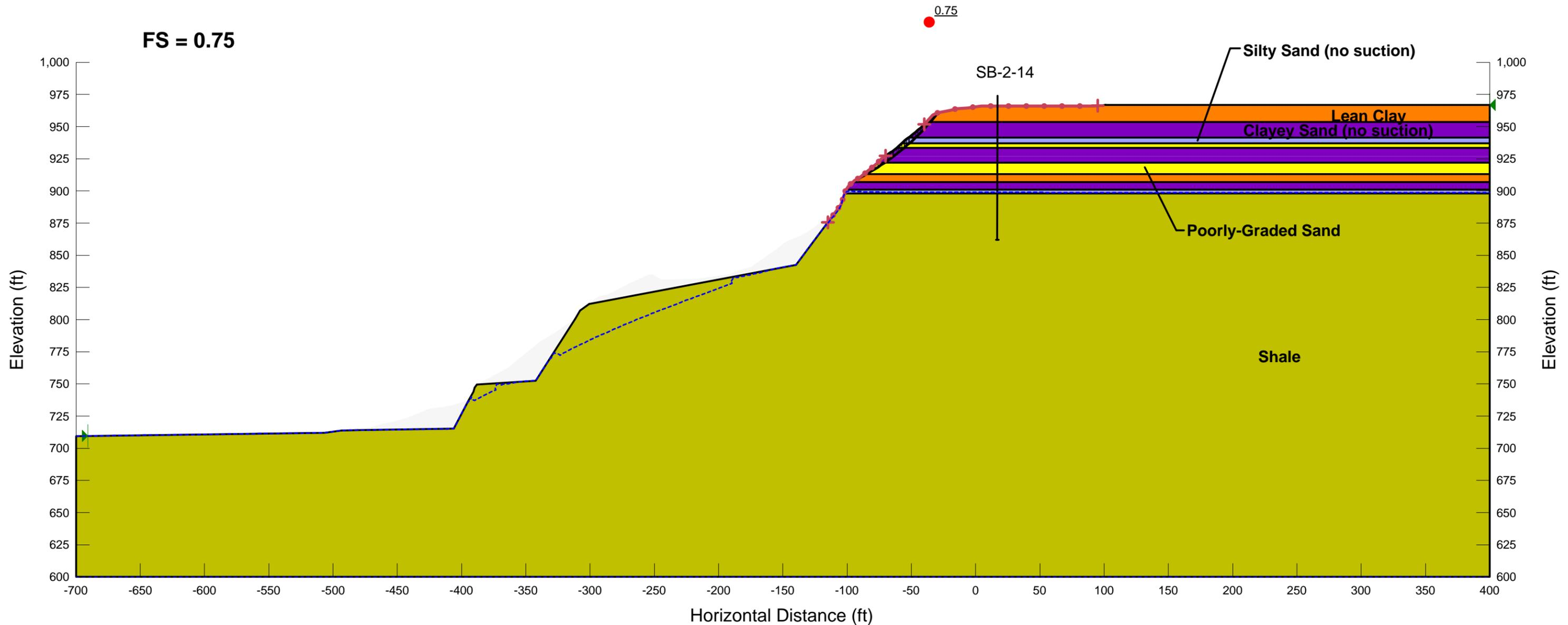
**Figure E-5 North End Drained Friction Angle with Suction with Rainfall**
