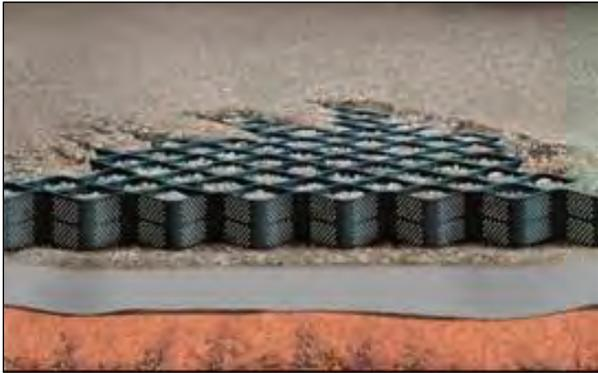
Photo 5-5 Cross section view of Geoweb (Source: [www.prestogeo.com](http://www.prestogeo.com), used with permission)
