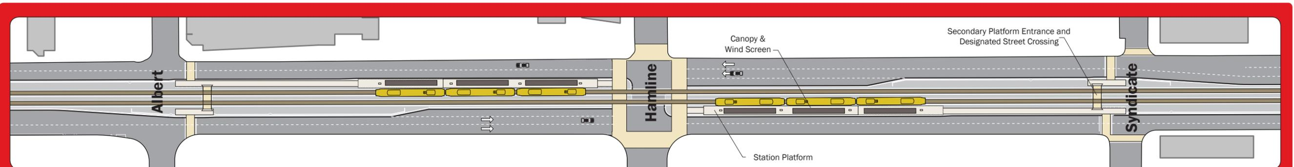
**FIGURE 2.1 - The diagram above represents a typical split side platform as it might look within the future Hamline Station Area**
