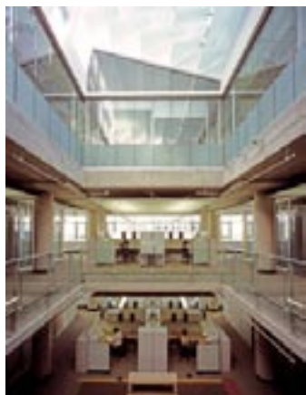
An extensive daylighting system reduces the need for electric lighting.
