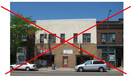
The cornice was removed during a remodeling many years ago and broke the cornice line with the adjacent buildings.
