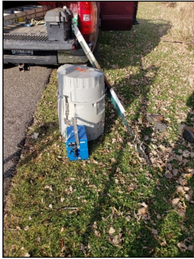
Photo 2-5: ISCO 6712 Sampler at Battle Creek
