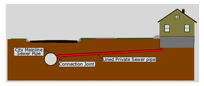
The City of Saint Paul's standard of repairing a defective connection joint is by digging and replacing the defective connection joint with a flexible tap saddle.
