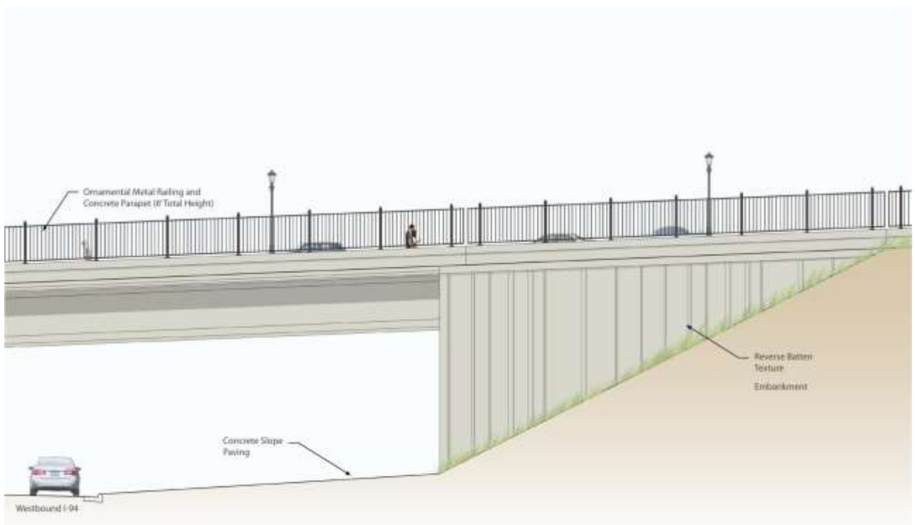
Proposed Bridge Abutment Side View
