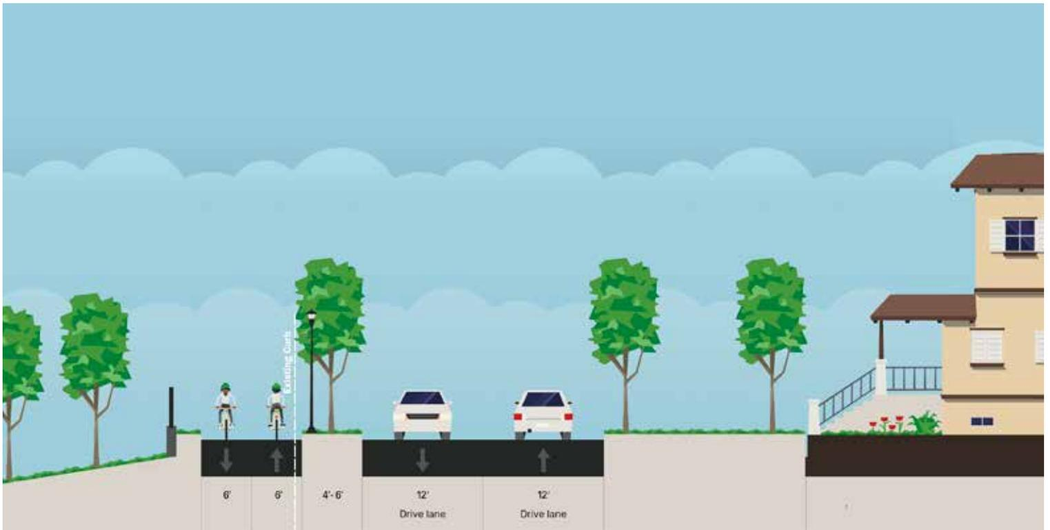
Figure 28: Segment 5B typical section south of Stinchfield St.
