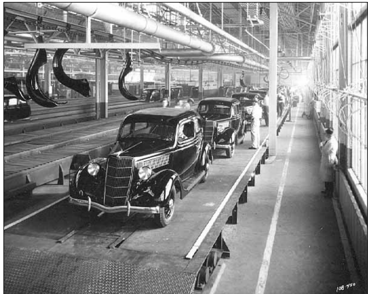
The exposed interior structure, pipes, and ductwork can be seen in this photograph of a finished car on the assembly line along the west wall of the plant, 1935. (Minnesota Historical Society)
