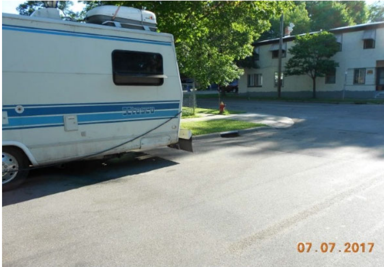
Sanitary Discharge to Storm Drain from RV 13
