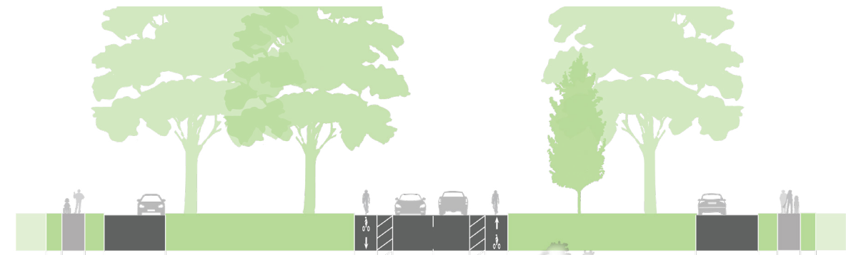
Fig. 3-28 | Typical 200-foot ROW with double median
