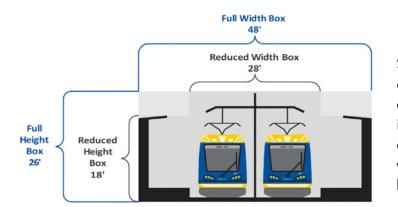
Space necessary for safe and efficient transit operations can be envisioned as a box or envelope around the transit components. The image shows various configurations for the transit envelope. Metro Transit staff are ready to work with a developer toward a creative solution that benefits the desired uses on the site.
