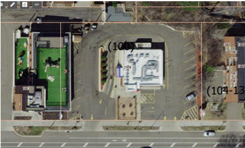
Above: 1959 Ford Pkwy is designed with additional pavement and a larger front yard setback to accommodate drive through vehicles. Zoned T2.
