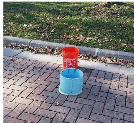
Photo 11-2: Victoria Street Infiltration Testing
