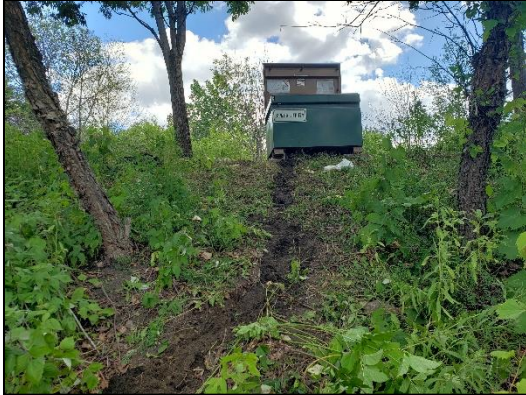
Photo 2-5: Job Box Housing ISCO 6712 Sampler
