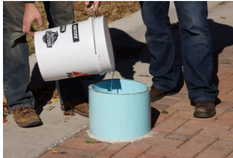
Photo 2-10: Permeable Pavement Infiltration Test
