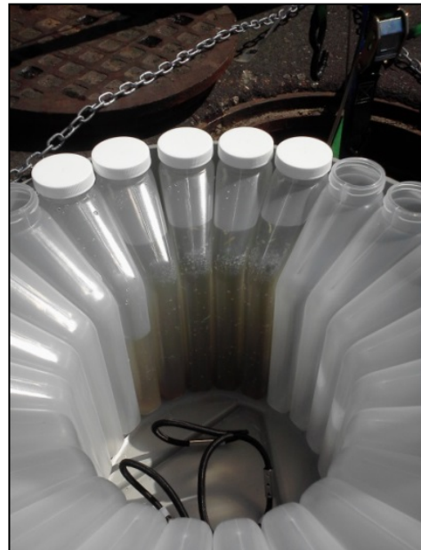
Photo 2-7: ISCO Bottle Configuration
