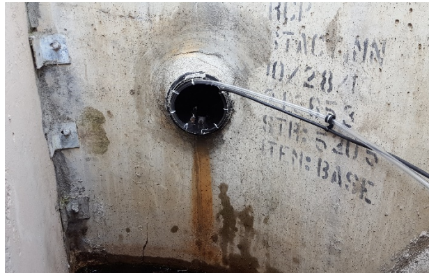
Photo 2-5: Sensor and sampler intake location in 8" drain tile in Magnolia Pond outlet control structure
