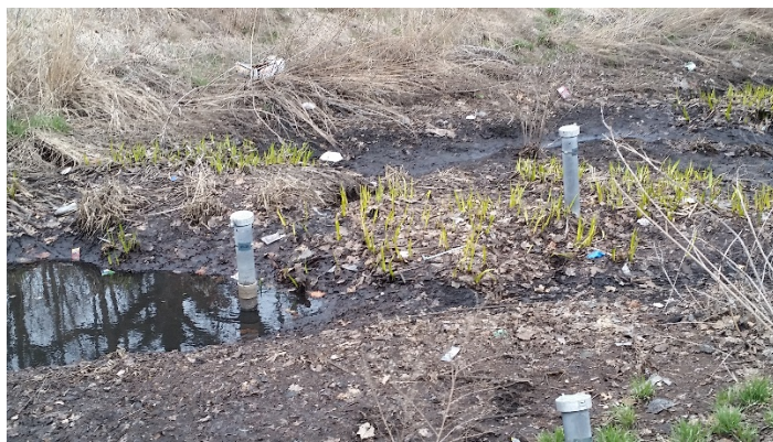
Photo 2-2: Beacon Bluff Rain Garden and in-rock permanent monitoring wells
