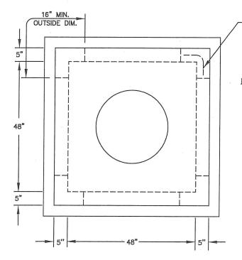
REINFORCING EXTENDING TO 1" MIN. CLR. AT CORNERS OR CONTINUOUS REINF. AROUND CORNERS
