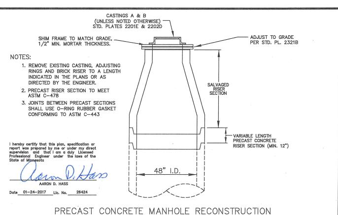
PRECAST CONCRETE MANHOLE RECONSTRUCTION (OR MANHOLE ADJUSTMENT OF 18" OR GREATER)
