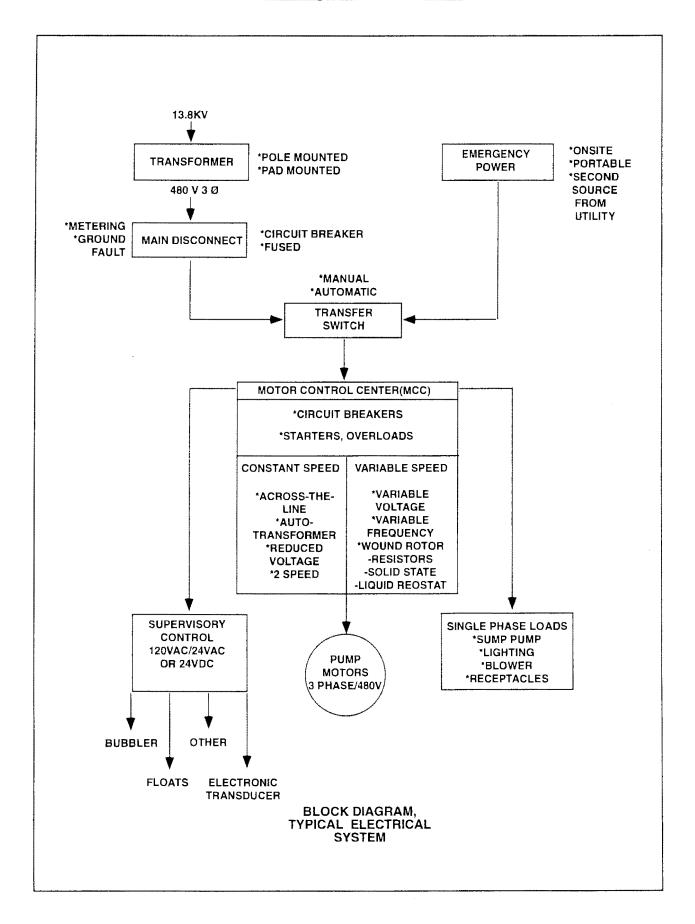
particular pump station the utility company transformer steps the voltage down to 480 volts, 3-phase.
