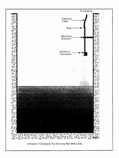
These systems are very flexible, easy to adjust and are consistent. Care must be taken, however, in their selection, installation and maintenance since microprocessors are susceptible to voltage surges on the line from lightning strikes, utility company switching and power failures.
