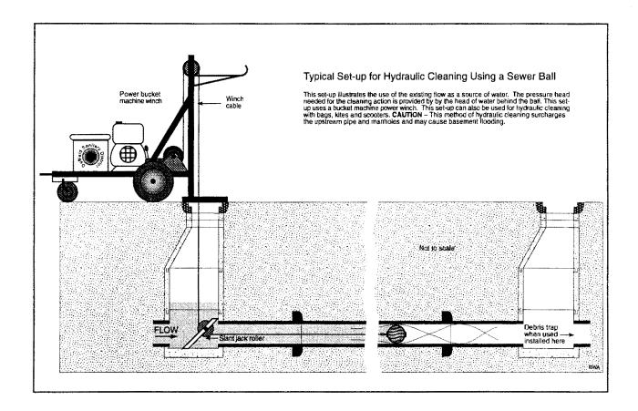
Balling is most commonly used in preventive maintenance programs. Under these conditions balling is very effective in reducing the possibility of stoppages developing.
