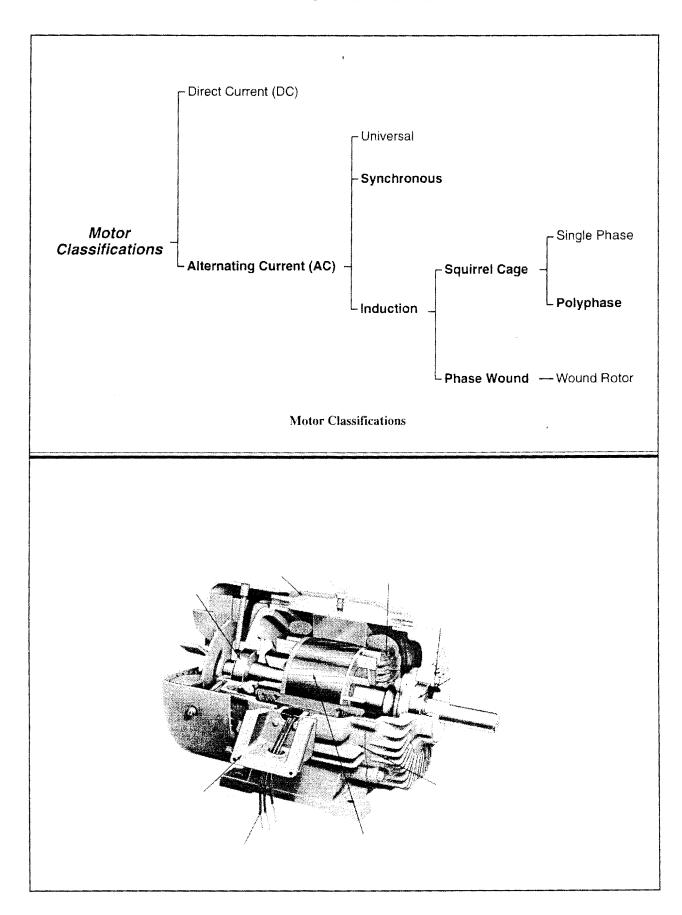
allows the external connection of various values of resistance. This causes the rotor to change speed ranging from zero RPM when the rotor circuit is "open circuited" to full RPM when the rotor circuit is "short circuited."
