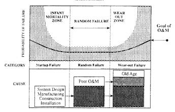
The probability of failures occurring is high during start-up, stabilizes once into the O&M period and begins to increase as the useful life is reached. Start-up failures are caused by errors in:
