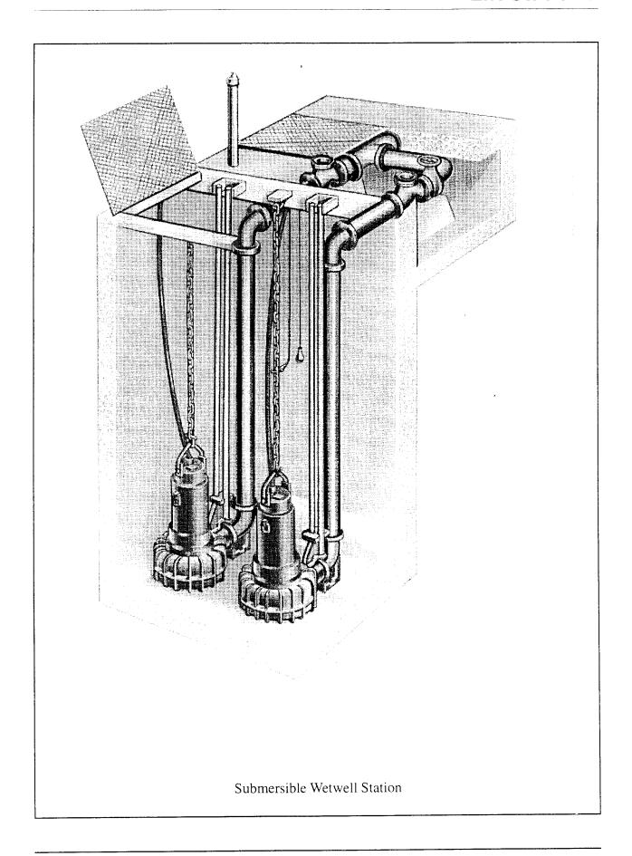
The weight of the pump keeps it in place and there are no bolts to remove.
