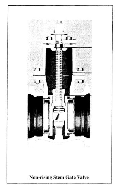
shaft into the flow area, the wedges slide against each other and provide wedging pressure on the back of the discs, which then seat against machined faces in the valve body.
