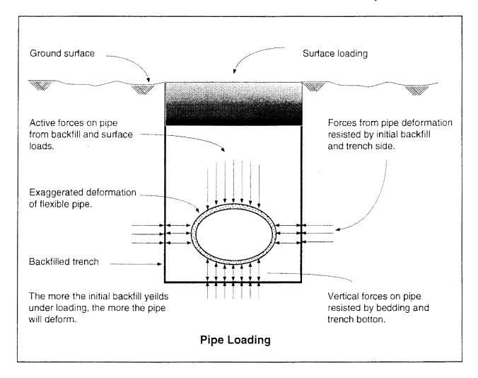
they convey, strength to withstand earth and surface loads, resistance to root intrusion, their ability to minimize infiltration and exfiltration, and the cost of the materials and their installation.
