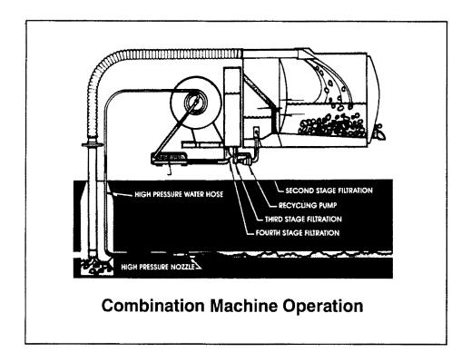
The recycling rate is faster than the water usage, assuring continuous sewer cleaning and eliminating trips to refill the water tank. The recycling system functions simultaneously or independently of the vacuum and water systems. Optional controls prevent the recycling pump from running dry. and the water tank from overfilling.
