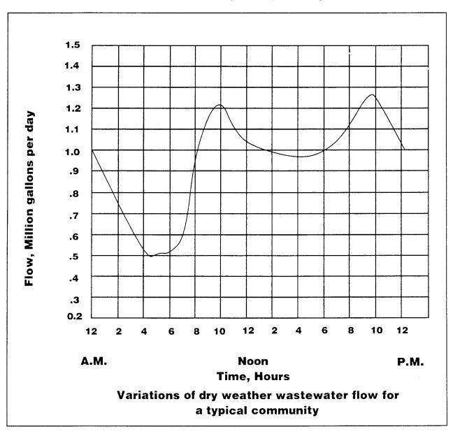
This type of graph which tracks the diurnal or daily flow changes as a function of time is a good diagnostic tool to determine the condition of the collection system and the amount of inflow or inflation occurring. If plotted on a frequent basis and analyzed, it would also provide indications of potential problems that have occurred such as a broken or collapsed line when significant variations from historical data is noticed.
