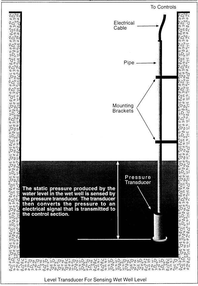
The microprocessor-based systems incorporate small computers into the supervisory control system. They can receive input from a bubbler-type wet well sensing system that translates air pressure into an electrical signal, from an electronic transducer mounted in the wet well or an ultrasonic level sensor.
