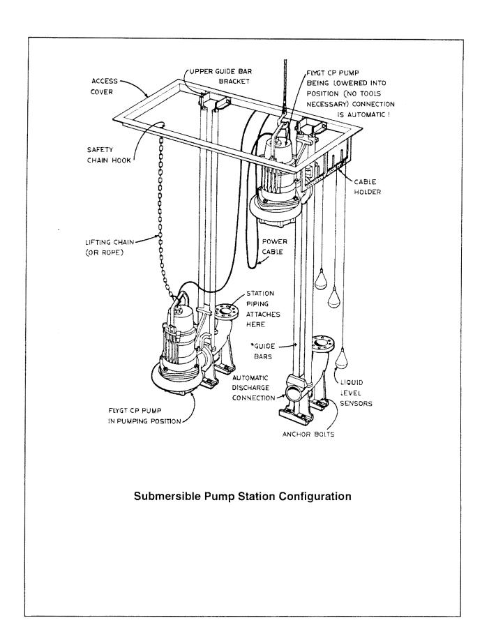
Equipment located in the wet well should be minimized, including suction and discharge valves, check valves, or other equipment which requires routine, periodic maintenance. This equipment can be located in small equipment manholes located adjacent to the wet well to make accessibility and maintenance much easier for the operator.
