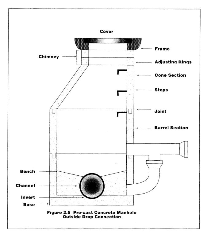
Manhole Material. Manhole bases are generally made of poured-in-place non-reinforced concrete with wastewater channels formed by hand before the concrete hardens.
