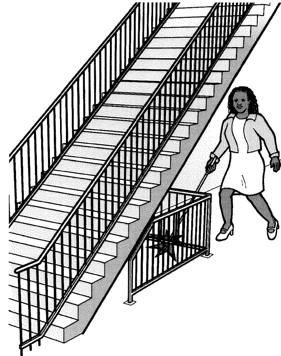
A detectable fence placed under this stair keeps people from running into the bottom of the open stair.
