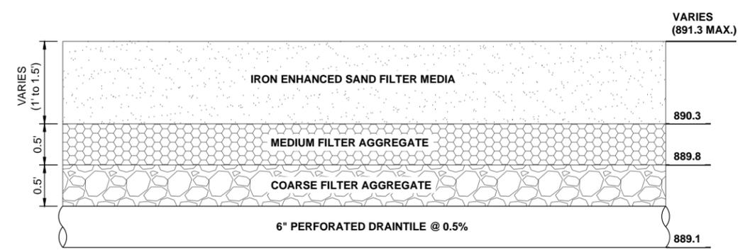
**IESF AGGREGATE GRADING LAYOUT (SECTION B-B)**
