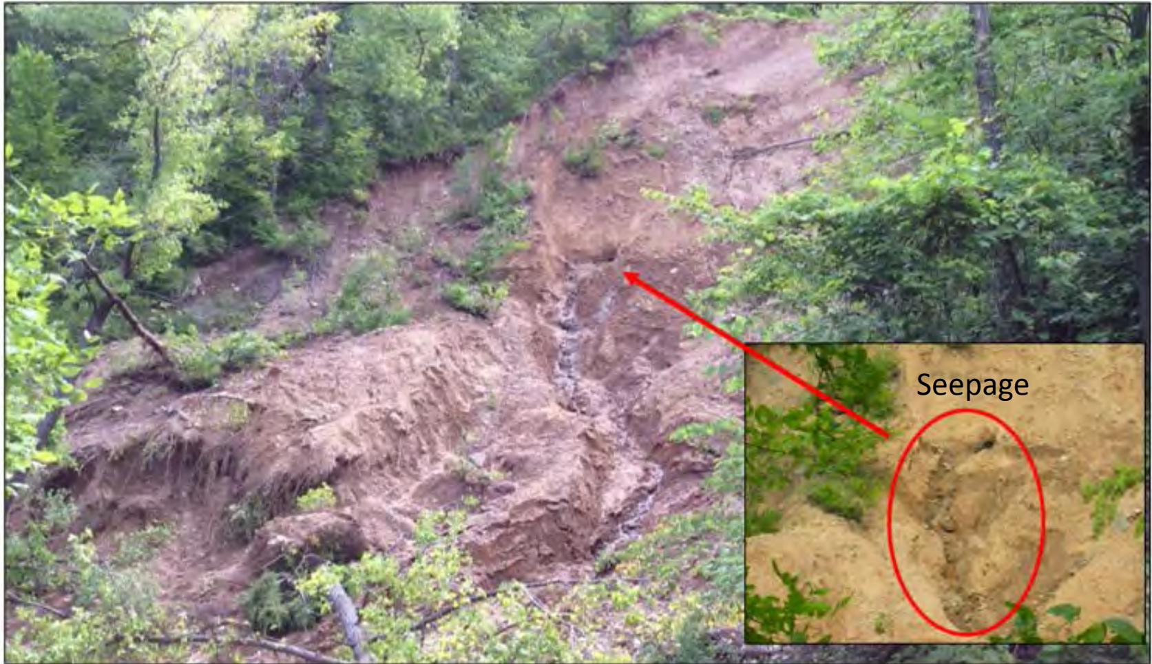
Large June 2014 slope failure from below with inset showing seepage (July 2014 site visit)
