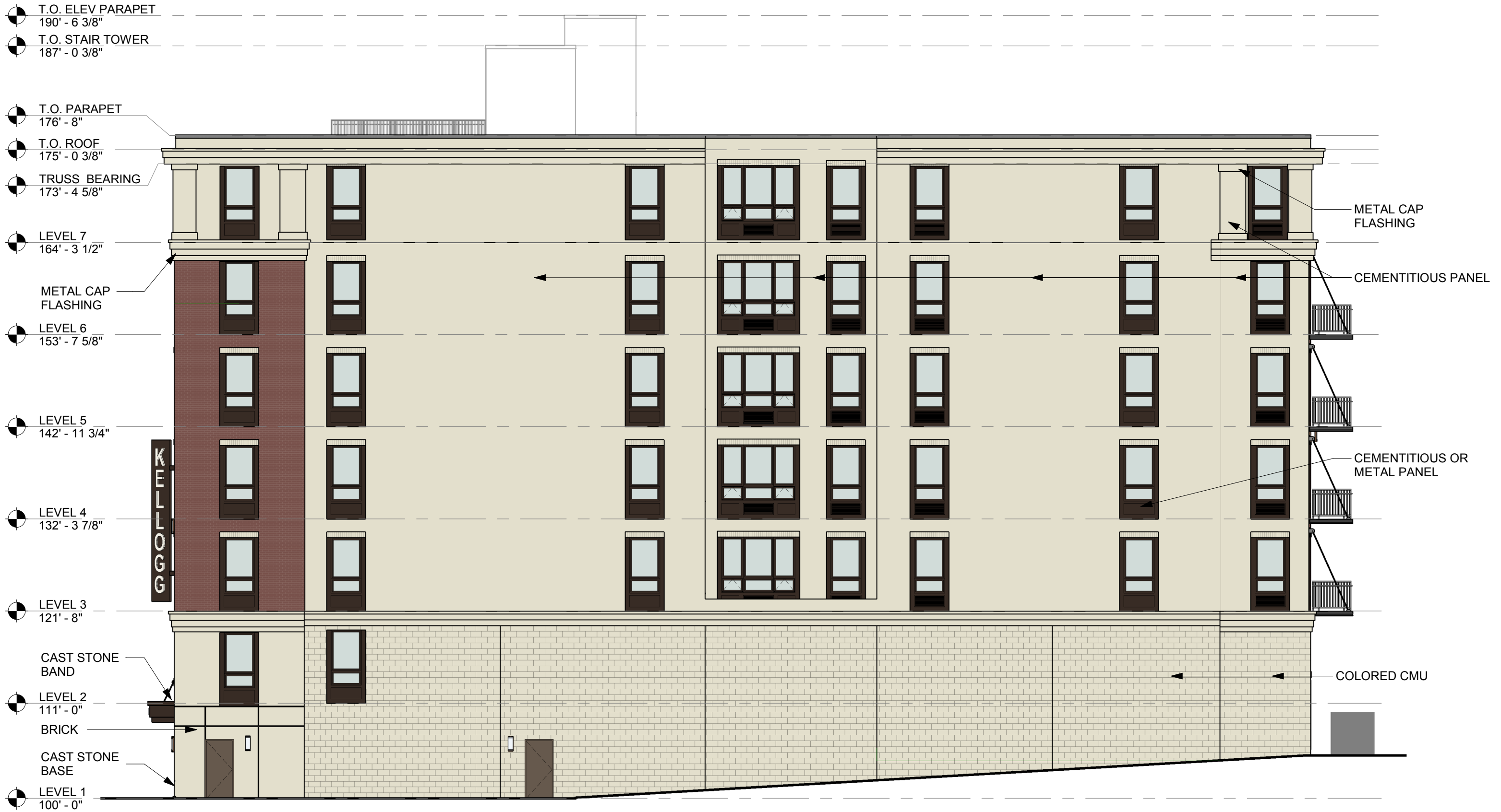
EAST EXTERIOR ELEVATION 3/32" = 1'-0"
