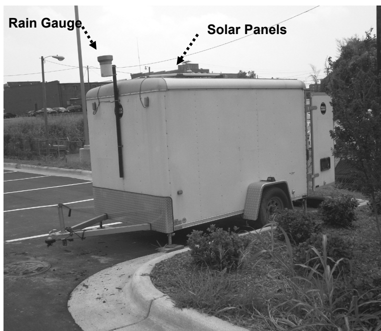
Figure 4. View of the Mobile Monitoring Unit (MMU) installed at the Mitchell Community College testing site.
