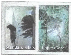
Impact resistance to wind-borne debris
