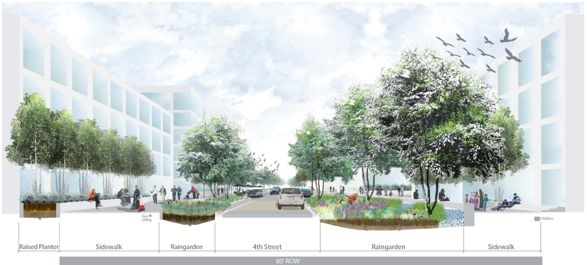
Figure 2.13 Boeser Concept: Illustrative Section Perspective- Overall Space Allocation
