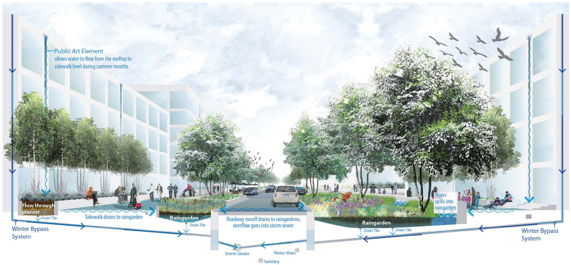
Figure 2.14 Boeser Concept: Illustrative Section Perspective- Stormwater Diagram
