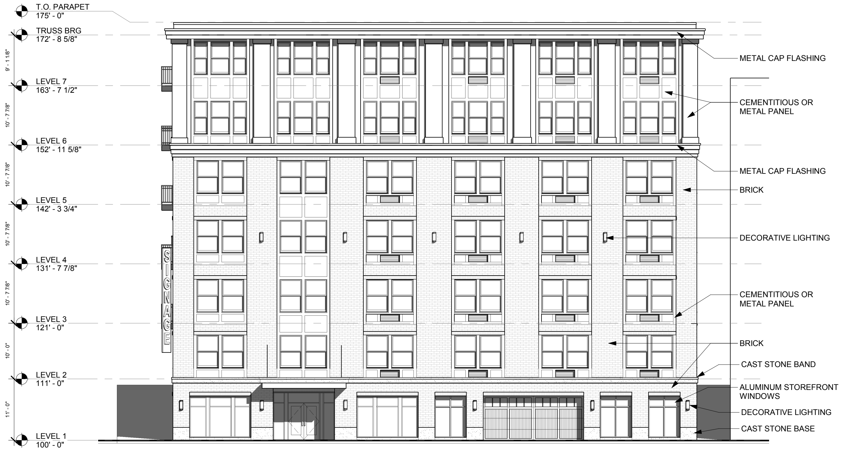
SOUTH EXTERIOR ELEVATION 3/32" = 1'-0"
