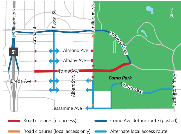
Como Avenue and Hamline Avenue intersection detour using Midway Parkway
