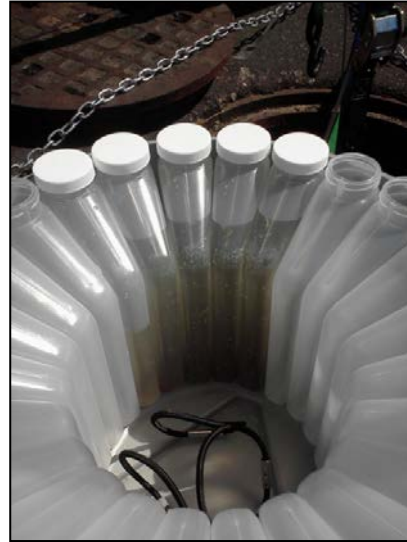
Photo 2-5 : ISCO 6712 sampling carousel (24 – 1,000 mL sample bottles)
