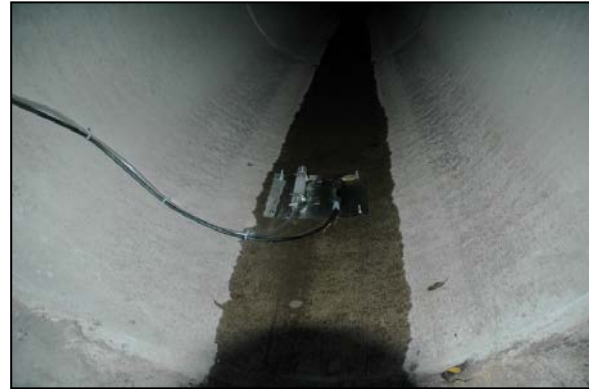
Photo 2-3: Flow sensor in upstream pipe in Beacon Bluff diversion structure
