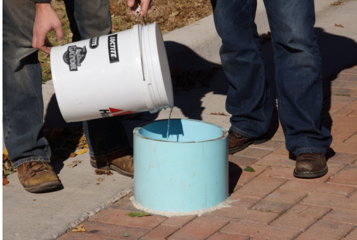
Photo 2-6: Permeable Pavement Infiltration Test
