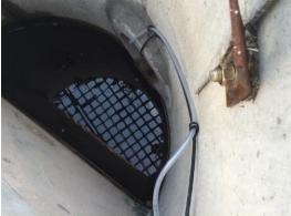
Photo 2-4: Flow sensor in outlet control structure Magnolia Pond
