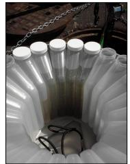
Photo 2-7 : ISCO 6712 sampling carrousel (24 – 1,000 mL sample bottles)
