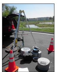
Photo 2-6: ISCO 6712 sampler at Beacon Bluff
