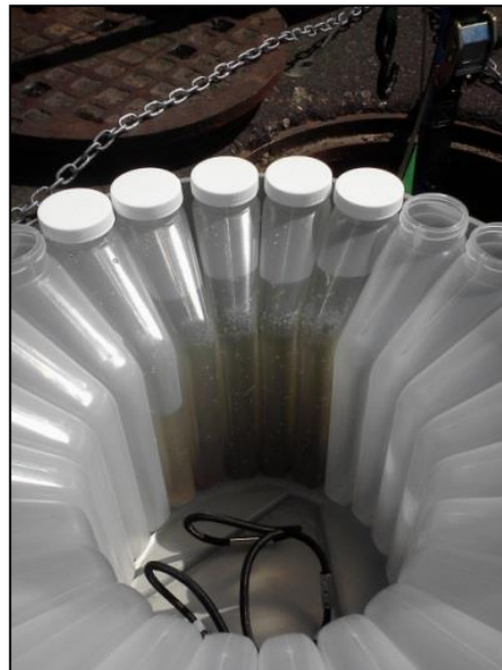
Photo 2-8: ISCO Bottle Configuration
