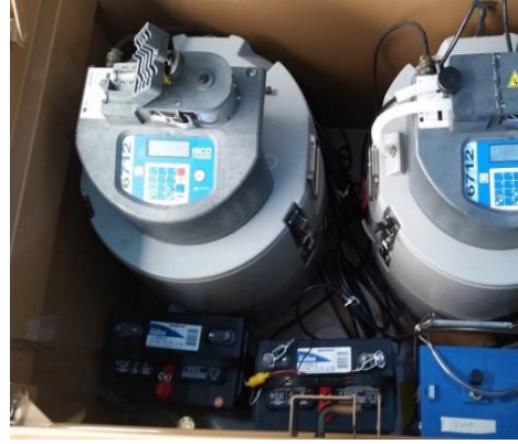
Photo 2-10: Maryland Pond sampler configuration
