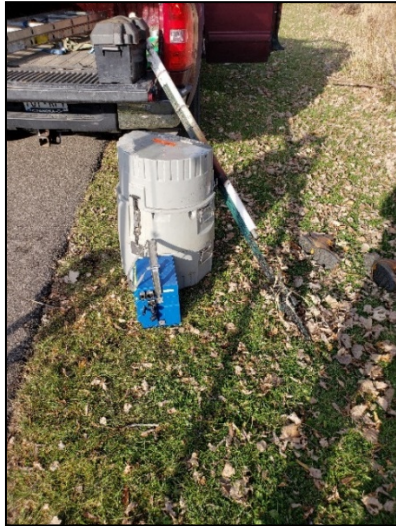
Photo 2-7: ISCO 6712 Sampler at Battle Creek
