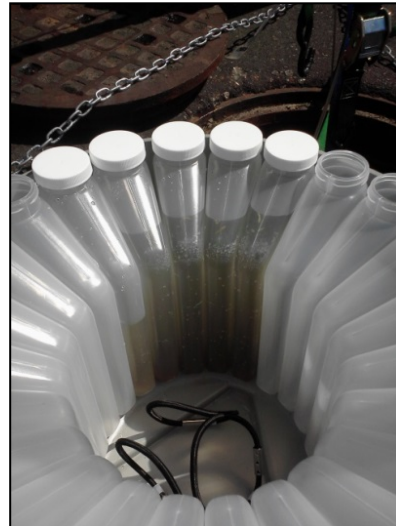
Photo 2-8: ISCO Bottle Configuration
