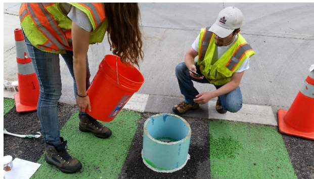
Photo 2-11: Permeable Pavement Infiltration Test
