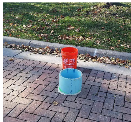
Photo 10-2: Victoria Street Infiltration Testing
