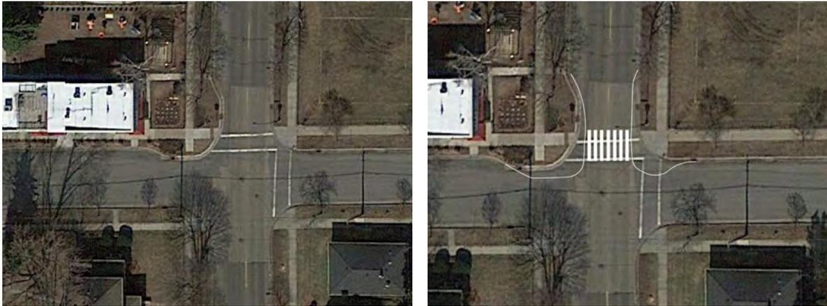
**Recommendations A.** Nebraska Ave and Hamline Ave. Current (left) and recommended (right). Installation of RRFBs, a high visibility crosswalk, vertical delineators, and on street paint will help to create a gateway to the area surrounding school.
