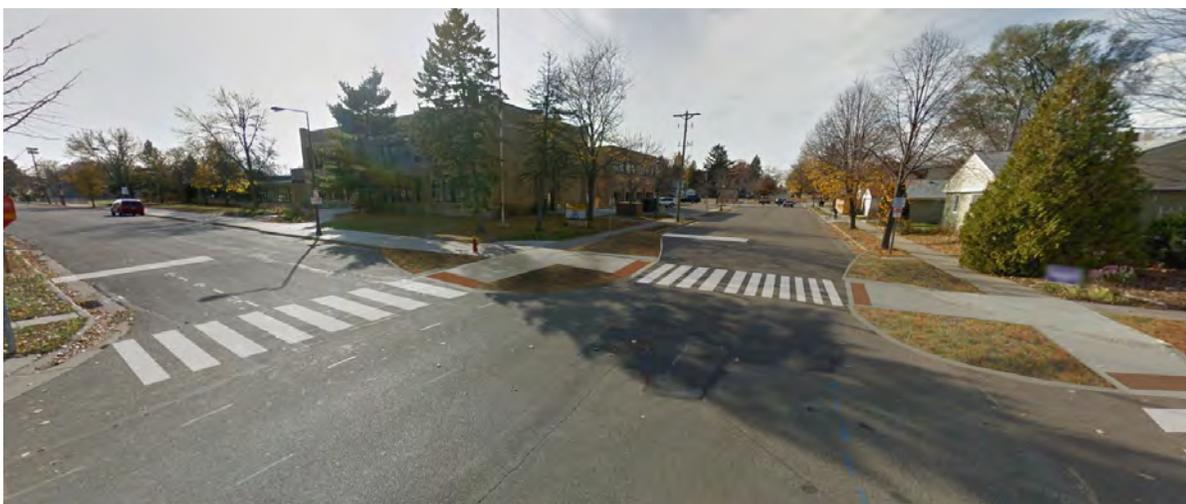
**Recommendation C.** Hoyt Ave and Huron St. Current (top) and recommended (bottom). High speeds of vehicles traveling on Hoyt Ave creates uncomfortable crossing for pedestrians. Installing curb extensions will shorten the crossing distance and decrease vehicle speeds.
