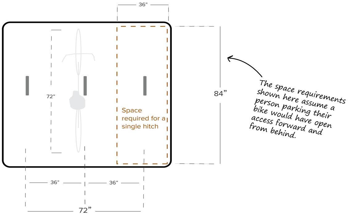
The space requirements shown here assume the area is confined on either side (left and right). Access is located at the top and bottom of the image, requiring a center aisle for circulation.
