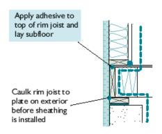
Alternatively, seal a strip of housewrap over exterior of rim joist, covering all joints, before sheathing is installed.
