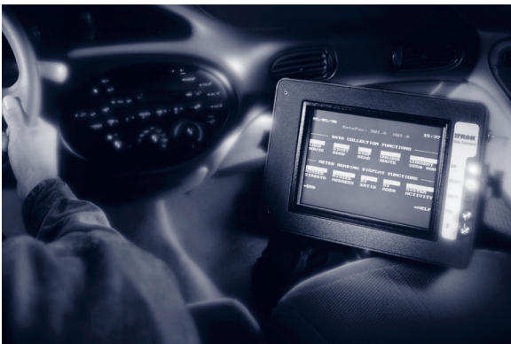
An electronic radio read system allows staff to obtain meter readings without entering the building. A monitor in the vehicle shows the water usage.
