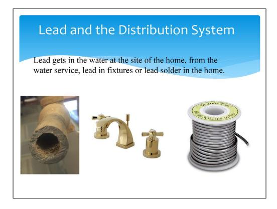
Lead can, however, enter the drinking water through lead service lines, brass fittings and fixtures and lead solder that was commonly used in private plumbing systems.
