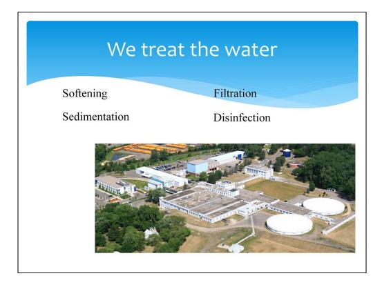
At McCarrons Treatment plant we treat the water to ensure it is of good quality and is safe to drink. To do this we first add chemicals to remove minerals and contaminants from the water, filter the water to remove even finer particles and finally, disinfect the water to ensure it contains no harmful bacteria or viruses.
