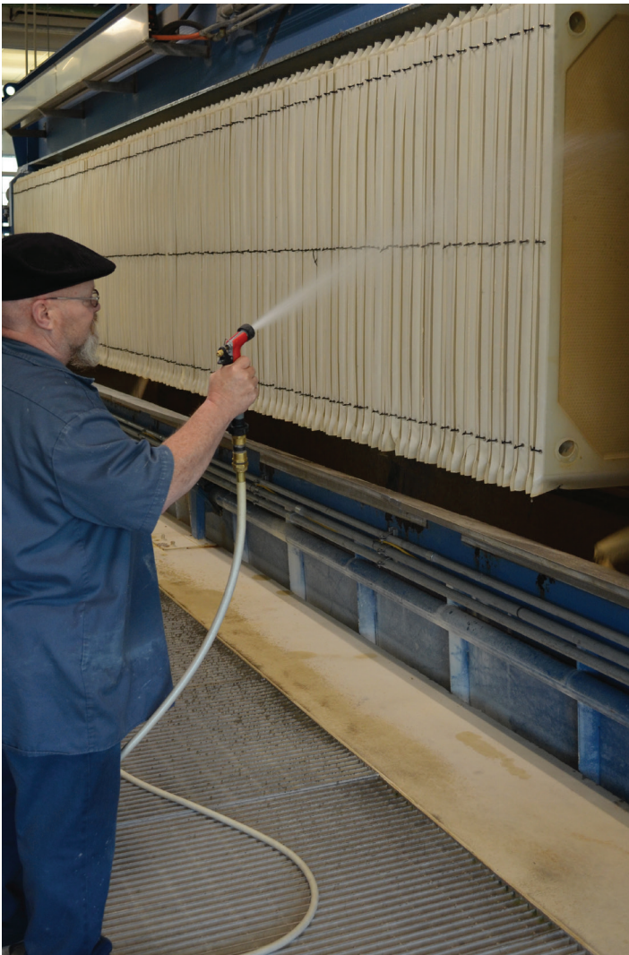
A worker cleans out the filters on a dewatering press.
