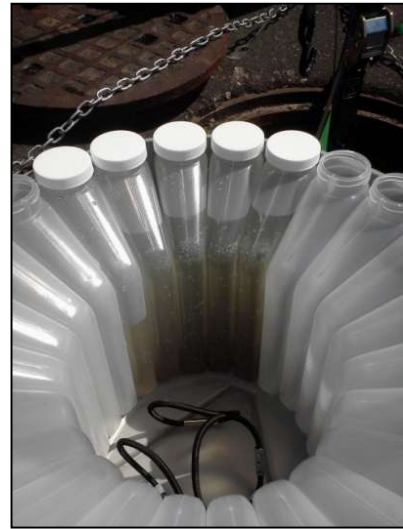
Photo 2-6: ISCO Bottle Configuration
