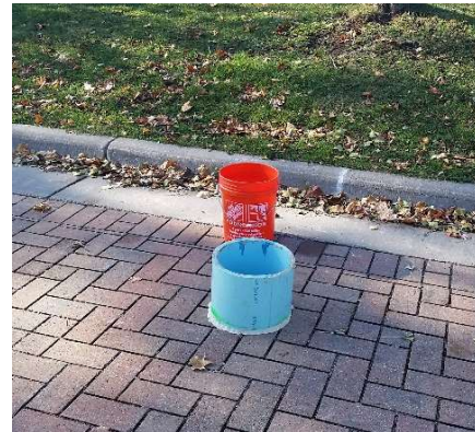
Photo 11-2: Victoria Street Infiltration Testing
