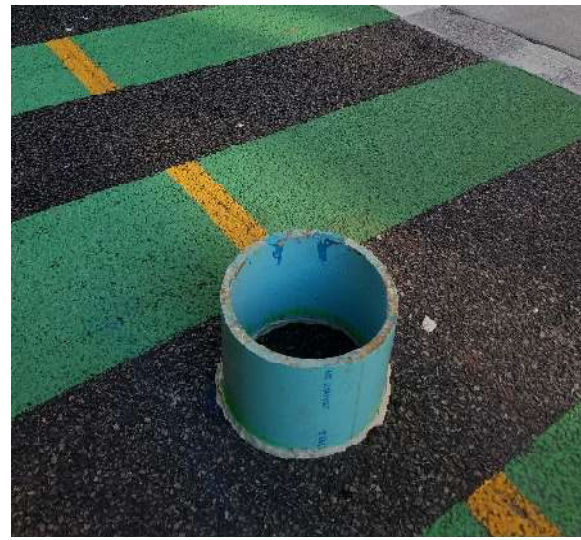
Photo 11-6: Jackson Street Infiltration Test
