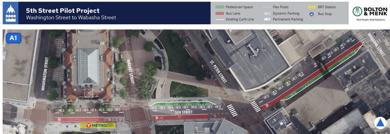
Figure 26 A one-block example of how the pilot project could be designed between Washington Street and St. Peter Street
